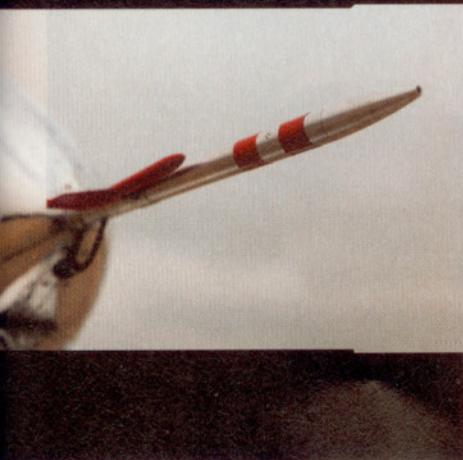
Back safely on the ground, they found the wings bent upward to angles of 18 and 23 degrees dihedral (the design angle was 5 degrees), and replaced them. The aircraft is one of a dozen BD-5Js still listed in the registry today.
